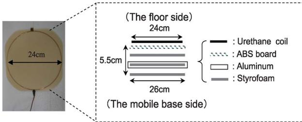
Fig. 2. Picture and structure of the antenna for 13.56 MHz.
