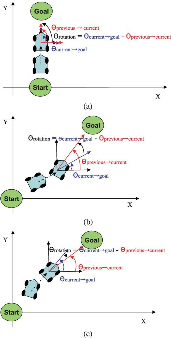
Fig. 9. Patterns of robot movement (a), (b), and (c). (a) Forward:  $\theta_{rotation} = 0$ . (b) Turn left:  $\theta_{rotation} > 0$ . (c) Turn right:  $\theta_{rotation} < 0$ .
